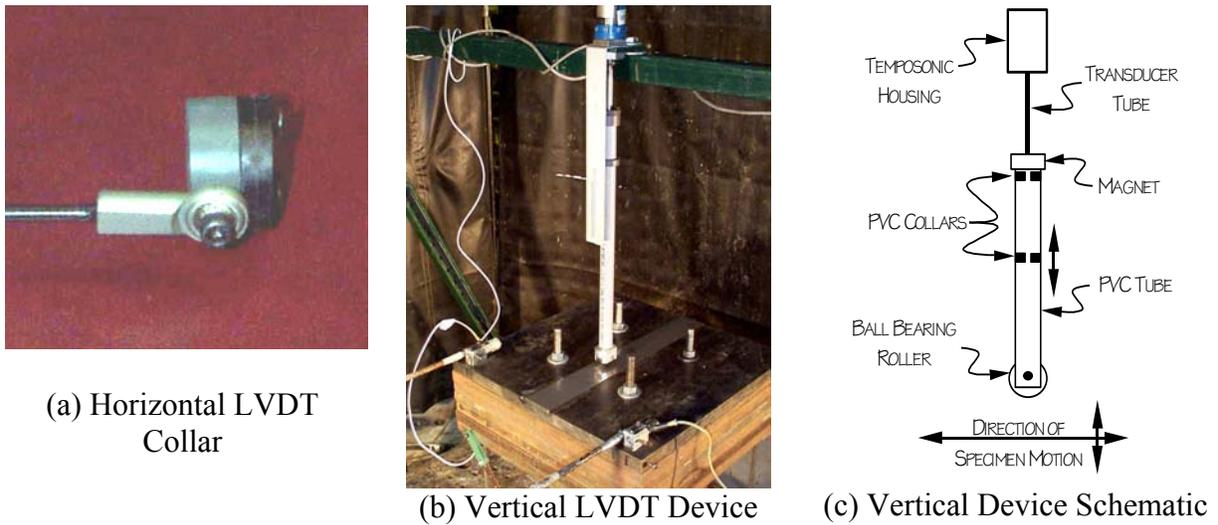
Figure 4: Displacement Transducer Modification Details
