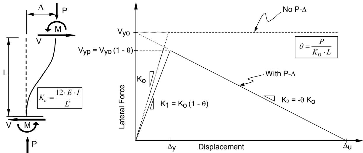
Figure 1: Free Body Diagrams of Typical SDOF structure
