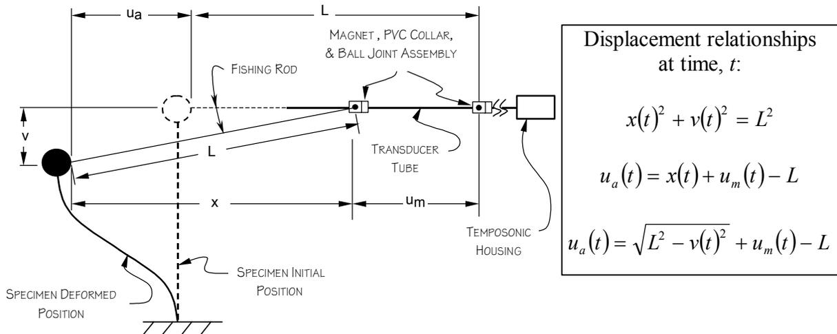
Figure 5: Definition of Variables used in Horizontal Displacement Correction
