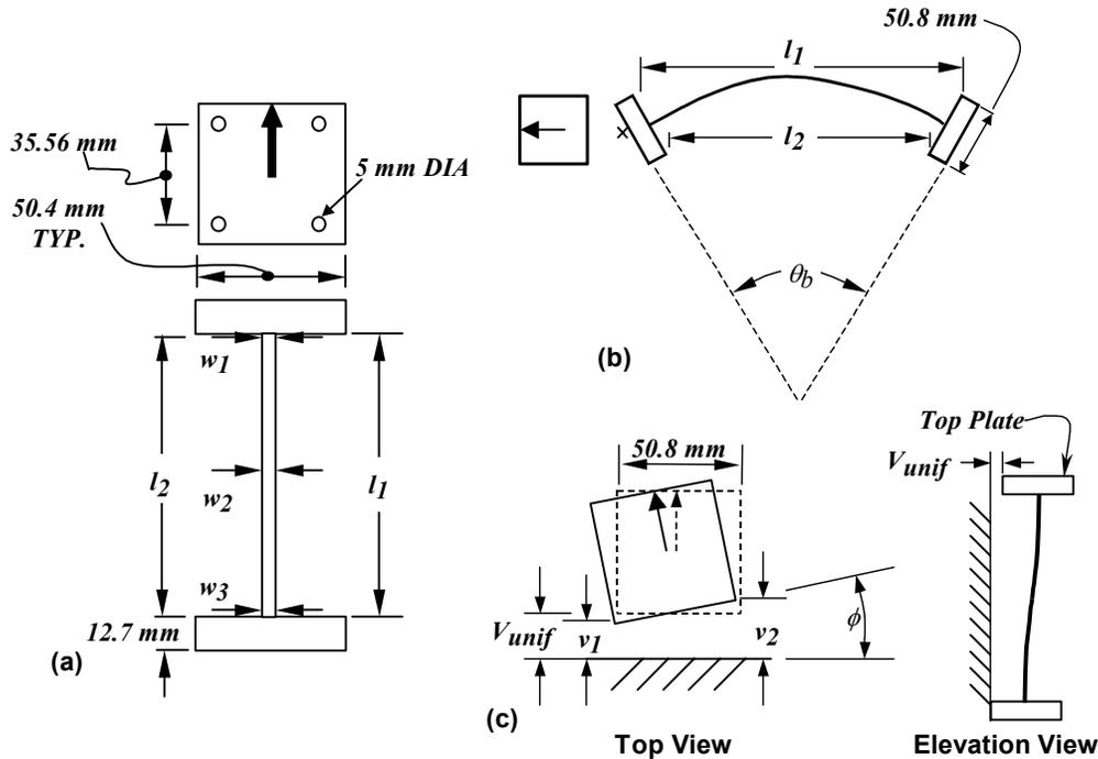
Figure 2: (a) Specimen Measurements in the U-D Orientation
