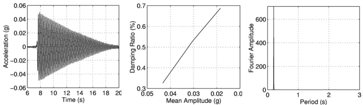
Figure 6: Free Vibration Test of Specimen 1 – AccWest Channel
